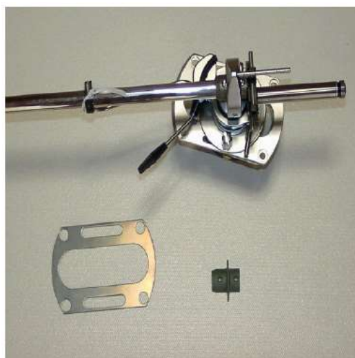
Figure 32 SME tone arm and improvement parts
